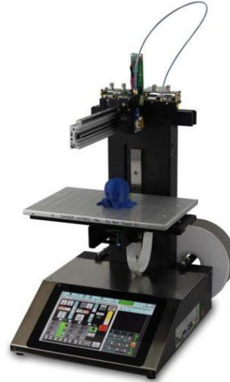
Figure 5-1: (left) Fused deposition modelling process invented by Scott Crump, comprised by a movable vertical platform (a) and two tempered extrusion printing heads for model (c) and support (d) feeding material contained on a feedstock spool (e). Both heads are allowed to move in XYZ (b) [13]. (right) Real example of 3D printer for FDM.
