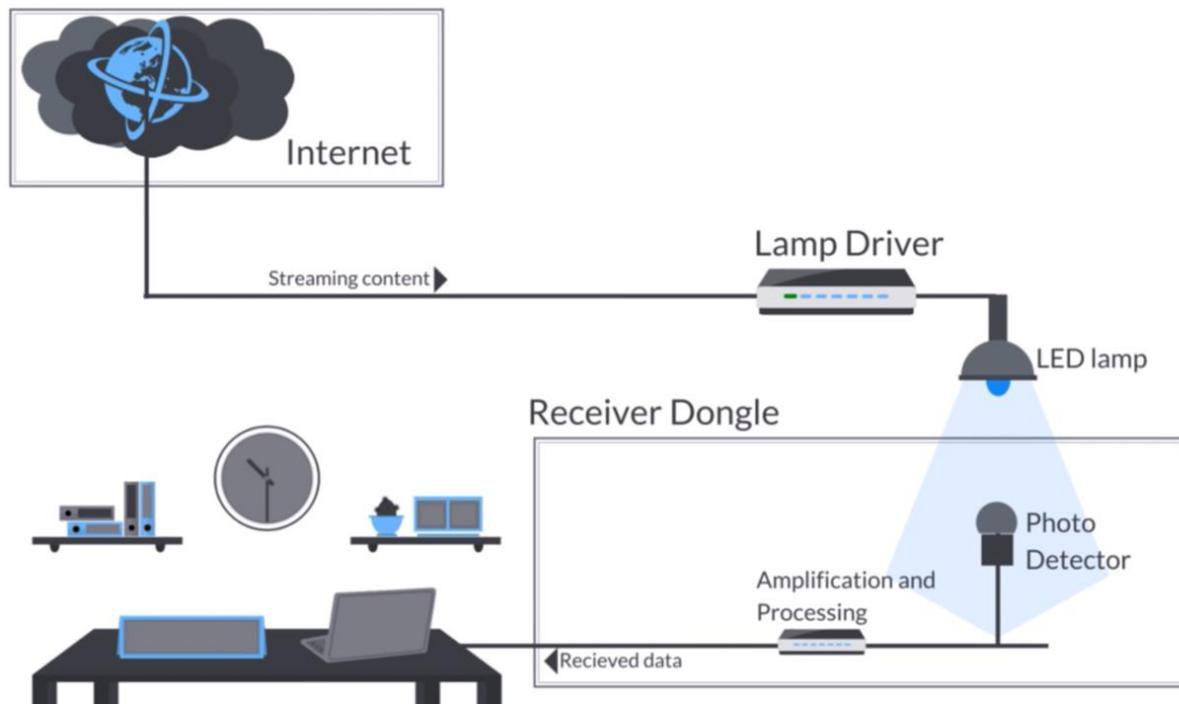
Figure 4.11 – Schematisation of data transmission through LiFi technology (Juice Tech Entertainment, 2016)
