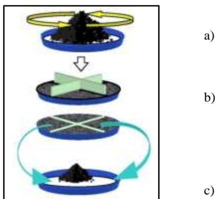
Figure 15. Homogenization (a), partitioning (b) and subsampling (c) procedures.
